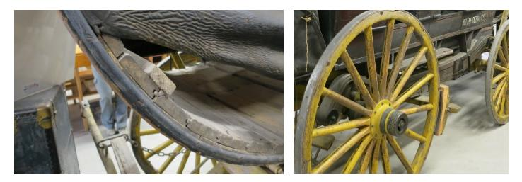
Well maybe there were. This photo on the left shows the joinery of the thoroughbraces. There is no turnbuckle. The thoroughbraces appear to have no splices. Comments?
